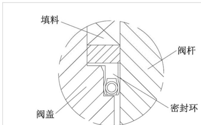
图7：双V形+翻边Lip-Seal结构组合密封 Figure 7: double-V shape + Lip-Seal structure combined seal structure
